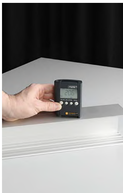
Schichtdickenmessung / coat thickness measuring
